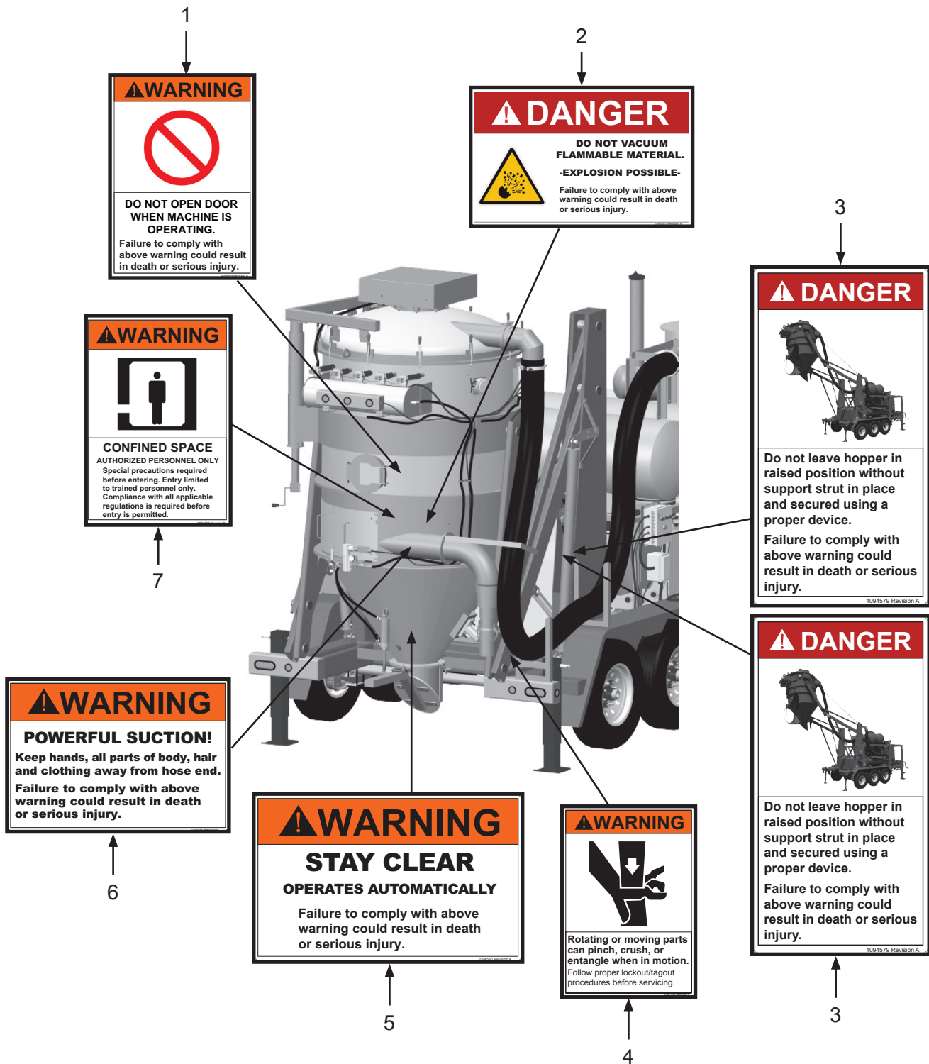
Figure 25: Hazard Identification Decals (Cont.)
