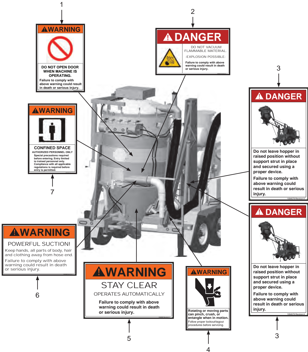
Figure 25: Hazard Identification Decals (Cont.)
