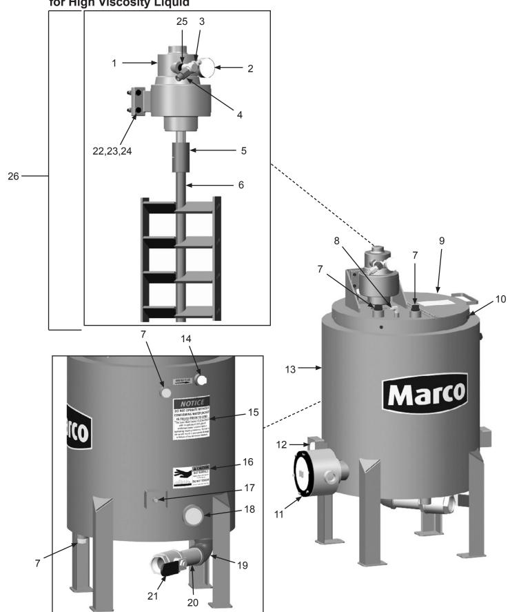
Figure 12: Spraymaster® 25 Gallon Heated Coatings Tank 240-Volts AC for High Viscosity Liquid with 5:1 Transfer Pump
