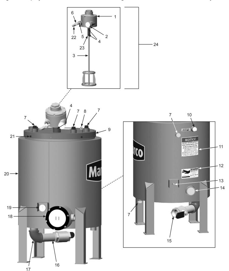
Figure 7: Spraymaster® 25 Gallon Tank 240-Volts AC Intrinsically Safe with 5:1 Transfer Pump
