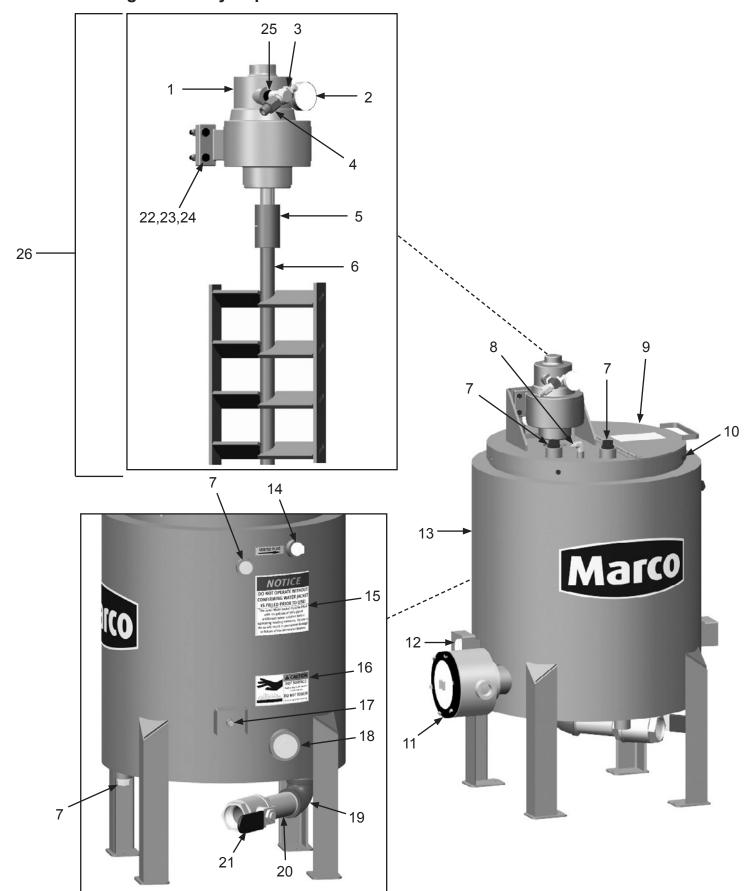
Figure 17: Spraymaster® 25 Gallon Heated Coatings Tank 240-Volts AC Intrinsically Safe for High Viscosity Liquid with 5:1 Transfer Pump
