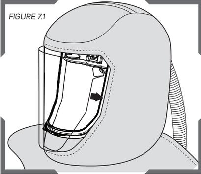
Peel off the backing of the cassette lenses and apply the lenses to the outside of the lens sewn into the hood.
