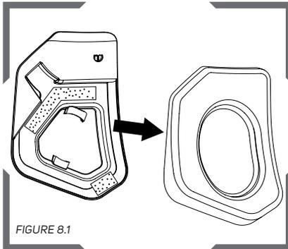
Remove the side pads from the covers that are attached with hook and loop.
