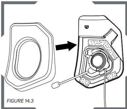
Attach the side pad back onto the cover over the Communication. Insert the side pad back into the helmet.
