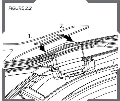
Line up the tabs of the lens with the clips on the sides of the helmet. 1. Slide the 1st side under the front side of the clip and slide back. 2. Snap the 2nd side of over the back of the clip.
