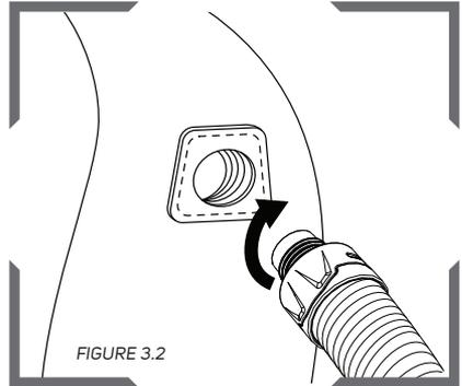
Insert the externally threaded end of the breathing tube into the inlet hole and tighten the breathing tube into the inlet until tight making sure not to twist the hood as it gets tight.
