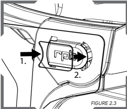
Do the same thing on the other side to fully secure the lens and the hood to the Helmet.
