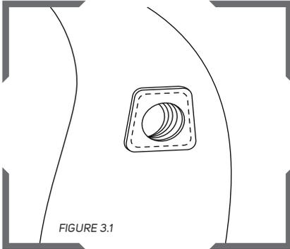
Line up the hole in the inlet seal with the inlet hole in the back of the helmet.
