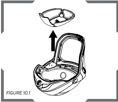
The comfort pad is attached to the inside of the Impact Liner with hook and loop. Pull the comfort pad out of the helmet.
