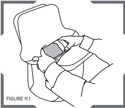
Open the bottom of the hood with the air flowing from the air source, put the respirator onto your head. Make sure the hood is centered on your head.
