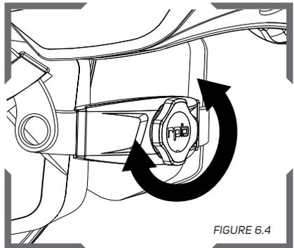
While wearing the T-LINK®, tighten the ratchet adjustment until the helmet and side pads sit comfortably on the head and ears.
