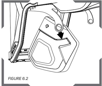
Slide the ends of the head harness into the slots on the side pad covers and reattach the head harness ratchet.
