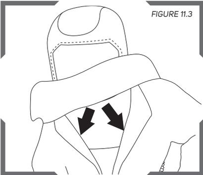
Tuck the inner bib into the collar of your shirt, coveralls, or protective gear to prevent contaminants from entering the hood. Pull the outer bib down.
