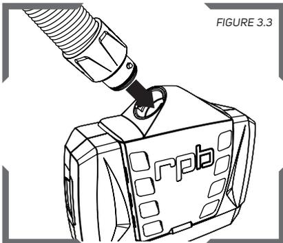
Insert the bayonet end of the breathing tube into the outlet of the PX4 AIR® PAPR and twist it in until it is secure.
