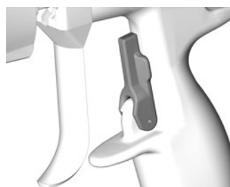
Gun Trigger Safety Unlocked
