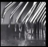
The bristles are obstructed (creating a tension), accelerated (released from the Accelerator Bar), impact the surface, and retract from the surface
