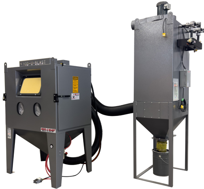
48" x 36" pressure-feed system, with 600 CFM Reclaimer , Reverse Pulse Dust Collector, and 1.0 Cu. Ft. Pressure Pot
