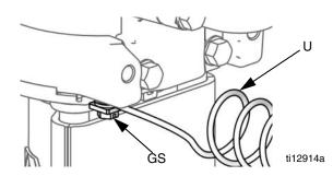
Fig. 2. Ground screw and wire
