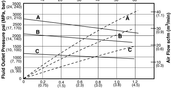
Fluid Flow gpm (lpm) tested in No. 10 weight oil
