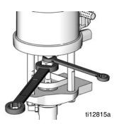
6. Lower the coupling nut (9) enough to remove the coupling collars (10), and then remove the coupling nut (9).
