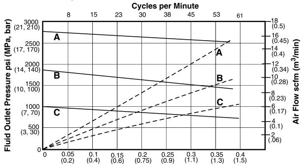
Fluid Flow gpm (lpm) tested in No. 10 weight oil
