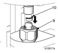
5. Screw the displacement pump into the adapter plate (3) until the cylinder top is flush with the top of the adapter plate.
