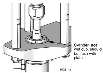
Fig. 6. Align cylinder and adapter plate.
