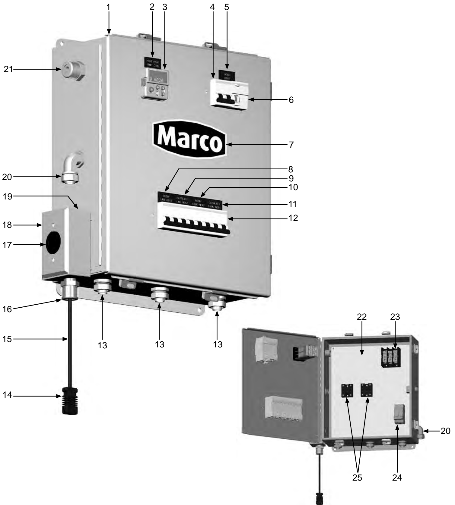
Figure 2: 240-Volt Control Box
