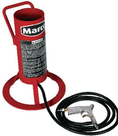
A suction blaster is a non-pressurized tank used to contain a supply of abrasive material for abrasive blasting. Used with a suction gun, the Blastmaster .20 Cu. Ft. Suction Blaster uses air pressure to move abrasive through an abrasive blasting hose and out the tip of the gun, producing a jet of abrasive. Typical applications include auto restoration, farm implements, hand tools, and lawn furniture. Common abrasives used include slags, glass bead, and mineral abrasives.
