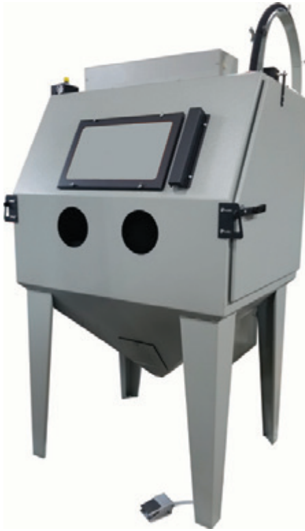
M44 Pressure-feed system with floating foot pedal
