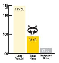
Blast Ninja<sup>™</sup> reduces nozzle air exit velocity while maintaining particle velocity – therefore reducing noise production at the source while maintaining blasting production. Oceanit performed many years of extensive fluid dynamic modeling, lab analysis, field trials, and rigorous operator testing in various conditions to arrive at the final Blast Ninja<sup>™</sup> product.
