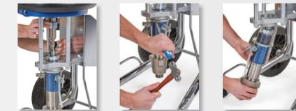
1. Remove rod coupling, inlet hose and paint hose
