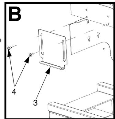
† Only used to mount hopper (8) on back of frame.
