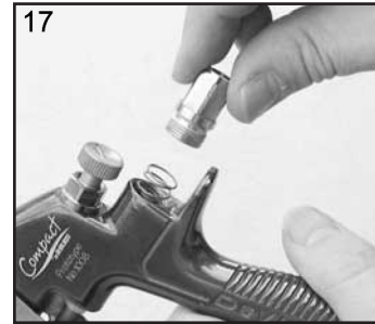
17. Replace Valve Spring and screw in Housing (10).
