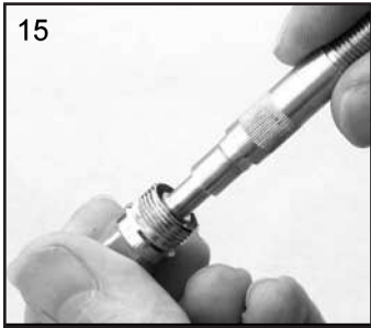
15. Fit Seal to Housing (10).
