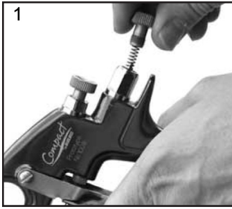
1. Remove Adjusting Knob (7), Spring (8), and Needle (9).
