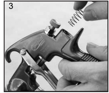
3. Remove Housing (10) and Air Valve Spring.
