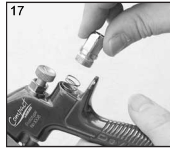
17. Replace Valve Spring and screw in Housing (10).
