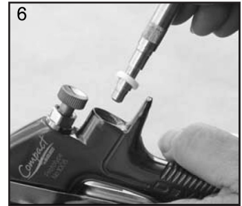
6. Remove Valve Seat.
