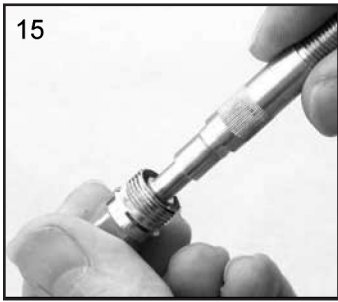
15. Fit Seal to Housing (10).
