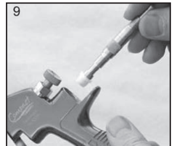
9. Fit New Front Seal to Service Tool.
