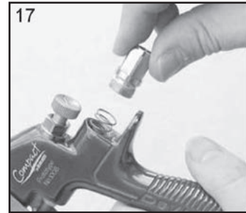
17. Replace Valve Spring and screw in Housing (10).
