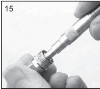
15. Fit Seal to Housing (10).
