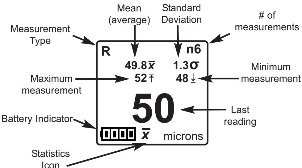
Remove the last measurement by pressing the (-) button. Press (+) to clear statistics.
