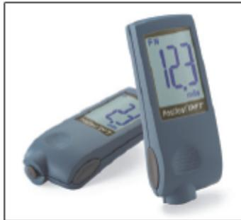
**Combo:** measures on all metals. The letter “F” (ferrous, e.g. steel) or “N” (non-ferrous, e.g. aluminum) is displayed with each reading depending on the substrate. Gage automatically recognizes the substrate.
