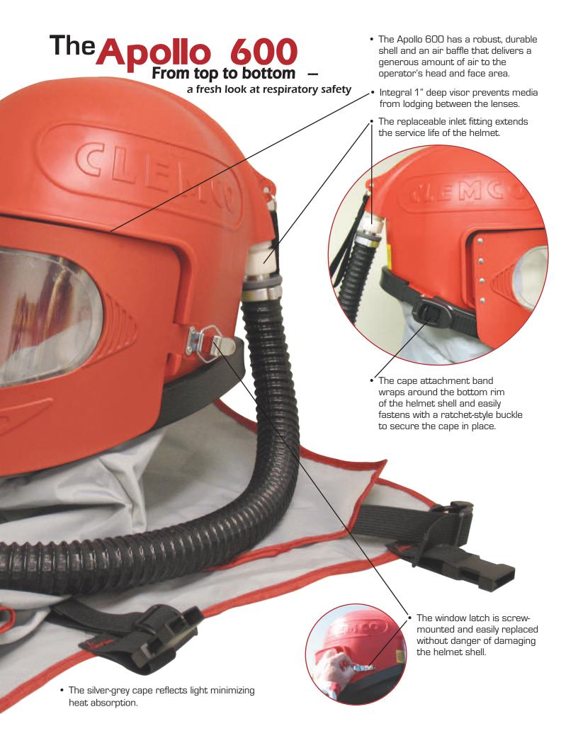
The Clemco Apollo 600 offers blast operators the very latest in respiratory safety and comfort. The 600 now is available with a choice of suspension systems—a DLX comfort-fit suspension, which provides a luxurious, cushioned fit around the head, or the classic-fit adjustable web suspension.
