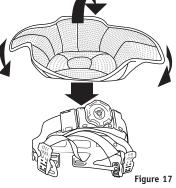
4) Fold the front-side flap over the suspension band and secure the fasteners to the outside material of the pad.
