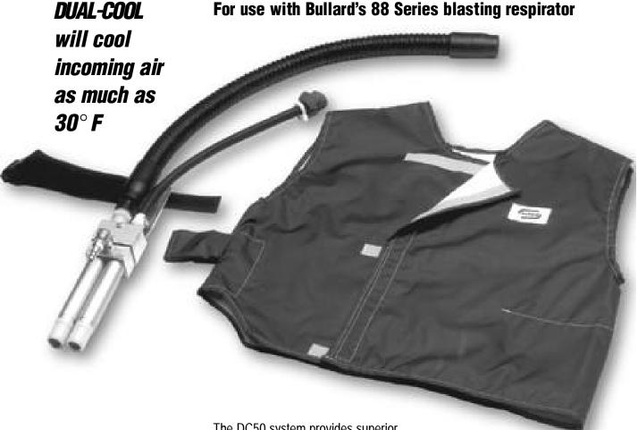
The DC50 system provides superior cooling to the 88 Series abrasive blasting helmet while also sending cool air to the vest for upper torso cooling. The DUAL-COOL will cool incoming air by as much as 30° F. The supplied-air system includes the DUAL-COOL tube, cooling vest, and breathing tube. The DC50 Series features separate air entry tubes to deliver air to the vest and to the breathing zone.
