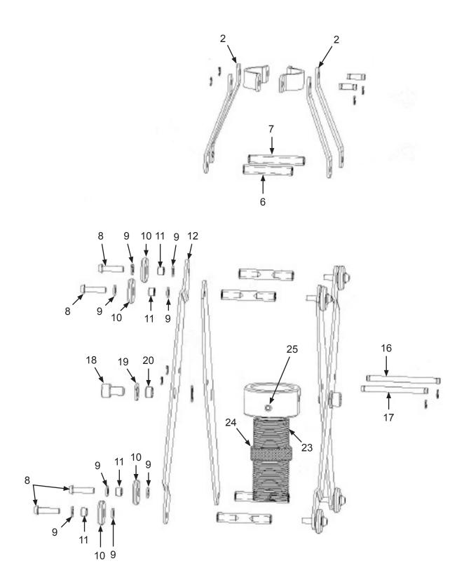
Figure 3: Internal Pipe Blasting Collar and Button Carriage System
