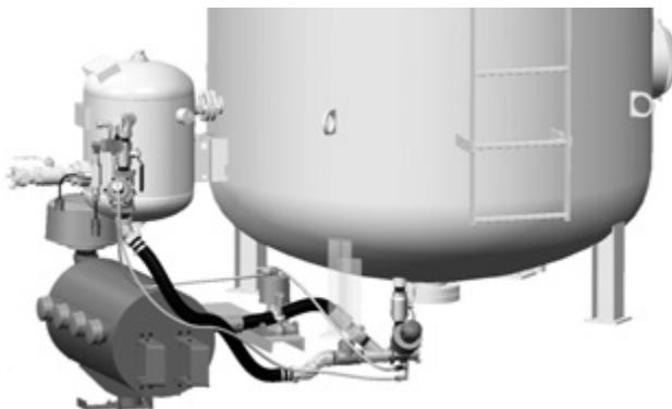
The Blastmaster® KwikStop Depressurization System quickly reduces the pressure from the blast hose when remote control switch is released. The abrasive-laden compressed air is exhausted into an expansion chamber where the abrasive is trapped and the air is vented to the atmosphere. This decreases the time required to remove pressure from the blast hose allowing the operator to reposition more quickly.
