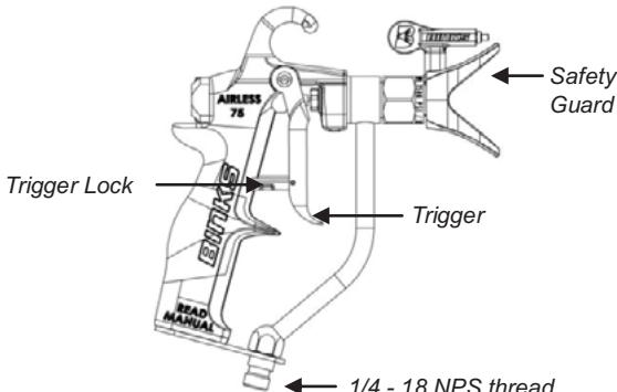
If you are using a genuine BINKS PIT BULL tip, follow the instructions below to install the guard and tip. If you are using a different tip, follow the installation instructions provided with the tip that you are using.
