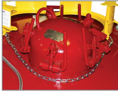
A chain allows the Pneumatic Closure Lockout Device to be retained near the camlock closure while loading the blast pot with abrasive.
