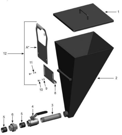
Figure 2: 15 Gallon Hopper – For Use With Cart Mounted Binks® Airless Spray Pumps
