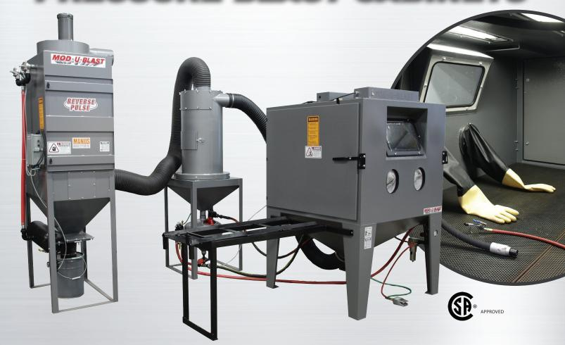
• **P-Series** blast cabinets are designed for use with: glass beads, glass grit, aluminum oxide, silicon carbide, mineral slags, or other blast media with a bulk density greater than 80 lb/ft and less than 130 lb/ft. PMB-Series and PSS-Series machines will accommodate lighter and heavier media's than mentioned above. Media type and size should be specified.
