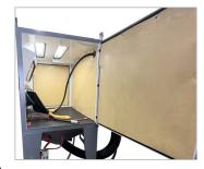
draping on sides and back of cabinet, H.D. rubber lined return hose, and tungsten carbide blast nozzle.
