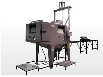
Custom direct pressure cabinet with two work stations, vertical door, external track system and pipe rolling cart.
