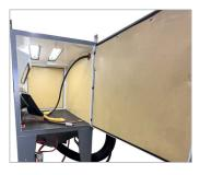
draping on sides and back of cabinet, H.D. rubber lined return hose, and tungsten carbide blast nozzle.
