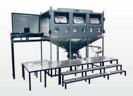
Custom direct pressure cabinet with 3 work stations, external track system, pipe pass through and pipe rolling cart.
