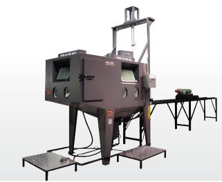
Custom direct pressure cabinet with two work stations, vertical door, external track system and pipe rolling cart.
