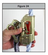
**Step 6:** The 8355 Fall Arrester is permanently connected to a SAL equipped with a self-closing and self-locking snap hook. Attach the snap hook to the dorsal D-ring of the FBH.
