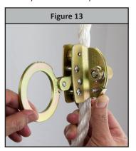
**Step 7:** Connect the SAL to the Arrester (if applicable).
