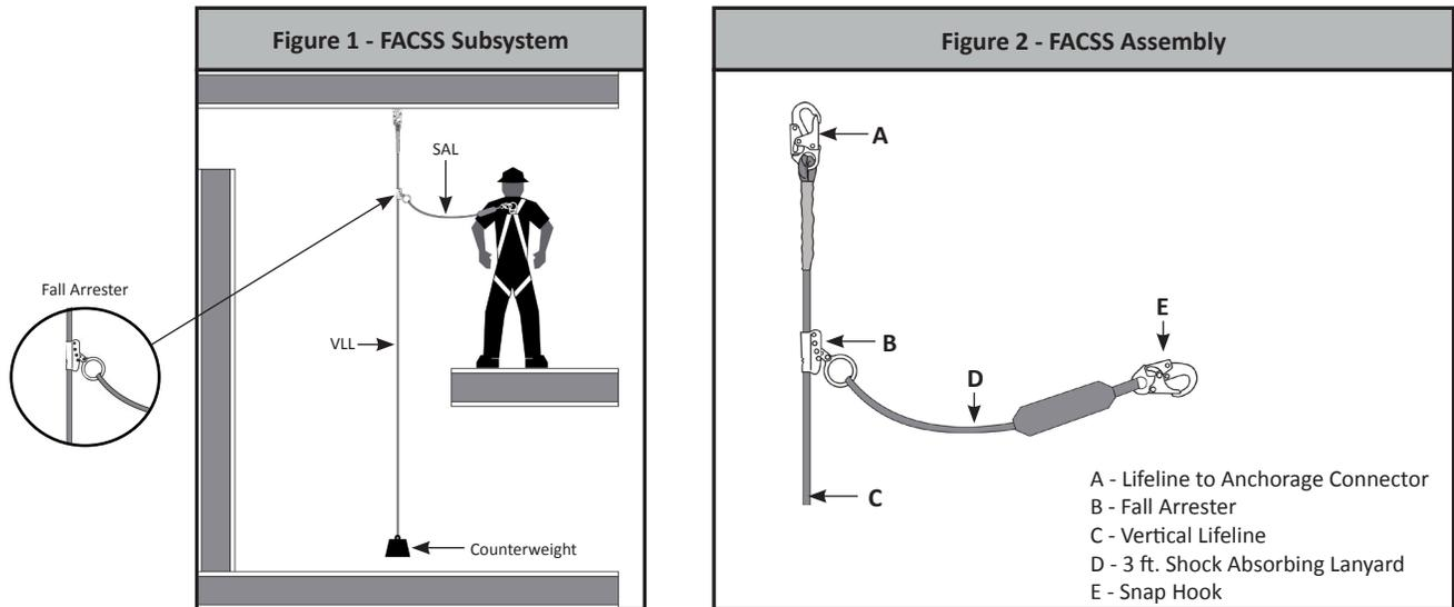
For the purposes of this manual, the system may be referred to as the equipment, Fall Arrester (Rope Grab), Fall Arrester Connector Subsystem (FACSS), the unit or the device. See Table 1 in Appendix A for ANSI/OSHA compliance information.
