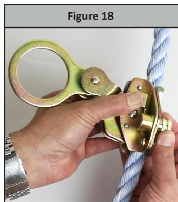
**Step 7:** Pull down on the ring and cam lever to ensure the Fall Arrester locks onto the VLL. These Fall Arresters are the trailing type. If a fall event occurs, the Fall Arrester will lock onto the VLL and arrest the fall.
