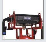
The Aftercooler motor and fan assembly allows for a large volume of air to pass over the aftercooler core, reducing the temperature of the incoming compressed air.
