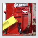
The reverse incline blade fan matched with the Baldor® motor produces up to 8,000 CFM of air flow, delivering optimal performance over other dust collectors in its class.
