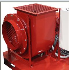
The reverse incline blade fan matched with the Baldor® motor produces up to 6,000 CFM of air flow at 2,800 RPM, delivering optimal performance over other dust collectors in its class.
