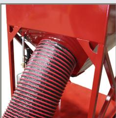
One 16" I.D. duct hose inlet port provides a large pathway for air to travel from a containment area.
