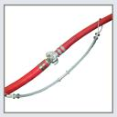
A Whip Check at each hose connection can prevent serious injury due to hose or coupling failure and meets OSHA requirements. (29 CFR 1926.302)
