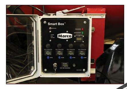
The Blastmaster<sup>®</sup> Smart Box Production Management System displays individual outlet daily production times, outlet 'in-use' indicators and total production time by outlet, for complete visibility on productivity.
