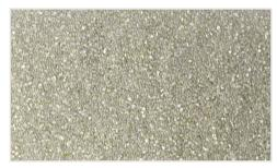
Glass Bead gently cleans metal parts without etching the surface, leaving a smooth, polished, or matte finish.
