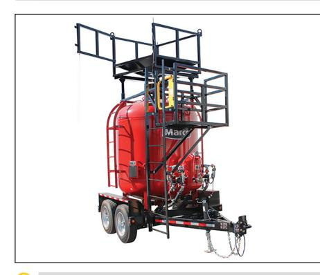
Blastmaster<sup>®</sup> Bulk Pot Platform mounts directly into the receiving collars located on the top of the Blastmaster 160 Cu. Ft. or 120 Cu. Ft. Abrasive Blasting Pot. The platform was designed to work primarily with the Blastmaster Heavy-Duty Bulk Bag Rack with Swing Gate, but can easily be used with any bulk bag rack with a 45" leg footprint. The Blastmaster Bulk Pot Platform provides an enclosed area to stand while accessing the top of a bulk pot.
