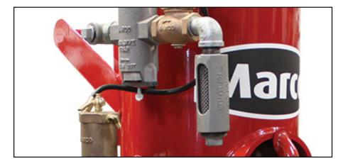
The Blastmaster® Abrasive Blasting Pot Muffler mounts vertically to ensure air and debris released during depressurization is exhausted away from workers. A muffler comes standard on all Blastmaster blast pots, reducing noise and trapping particles as they exit the exhaust port during the depressurization process.
