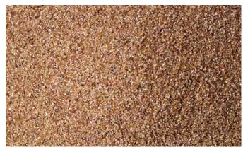
Alluvial Garnet has a sub-angular shape, hardness, and high bulk density, making it ideal for quickly removing thin to medium thickness coatings, mill scale, and rust. This lower-dusting abrasive naturally has low chloride levels, reducing surface contamination.
