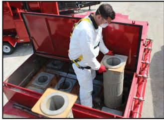
Dust collector filter cartridges trap dust particles removed by a dust collector system from abrasive blasting. High-quality filter cartridges are critical for keeping a dust collector operating effectively to maintain proper air flow and visibility on the work site. Marco offers dust collector filter cartridges that are high quality replacements for all major dust collector manufacturers.
