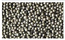
Carbon Steel Shot is a general-purpose abrasive used to remove mill scale and molding sand. Its high bulk density, low friability, consistent sizing, and low dust levels provide superior production rates.
