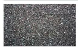
Aluminum Oxide is used when an application is sensitive to rusting caused by ferric contamination and requires an extremely aggressive, hard abrasive.
