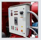
Easy-to-access control box with Emergency Stop Button for fast system shutdown.
